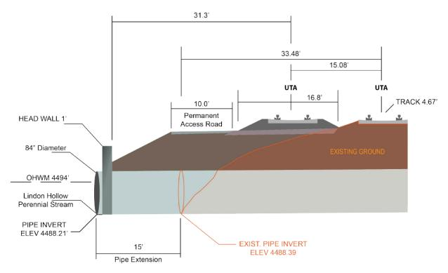
Cross-Section 2: Typical Cross-section with Permanent Access Road
